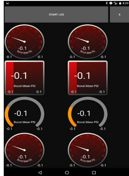
Automatic Logging on Full Throttle: this feature is exactly as it sounds. MHD logger will automatically begin logging once the Acc. Pedal reaches over 50% depression and stop the log when the Acc Pedal has remained below 50% for more than 3 seconds.. MHD will also PREPEND the 1 full second prior to the recording start so you see the full data in the log. Simply select "Monitor (Auto Logging)" from the Monitor tab to utilize this feature.
